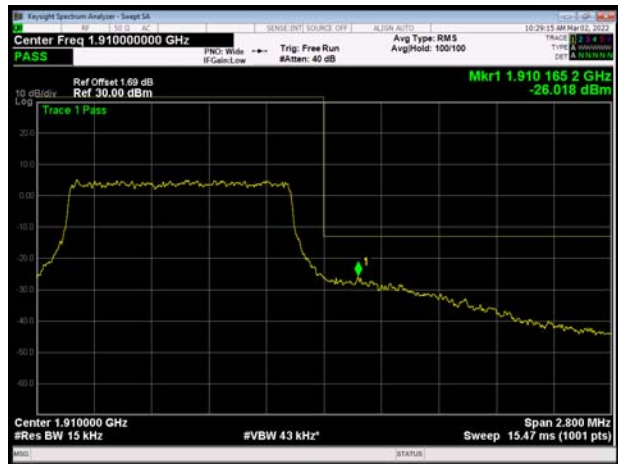
LTE Band 2 3MHz 16QAM 1RB CH-High
