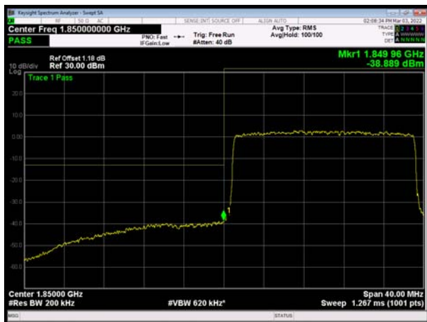
LTE Band 2 20MHz 64QAM 100%RB CH-Low
