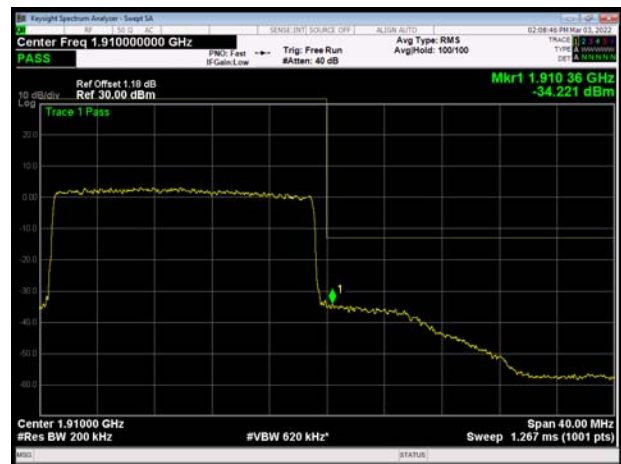
LTE Band 2 20MHz 64QAM 100%RB CH-High
