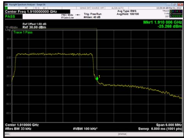
LTE Band 2 5MHz QPSK 1RB CH-High
