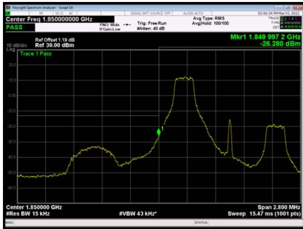
LTE Band 2 1.4MHz 64QAM 100%RB CH-Low
