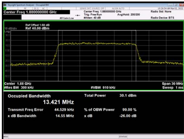
LTE Band 2 15MHz 16QAM CH-High
