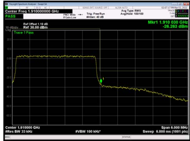
LTE Band 2 5MHz 64QAM 1RB CH-High
