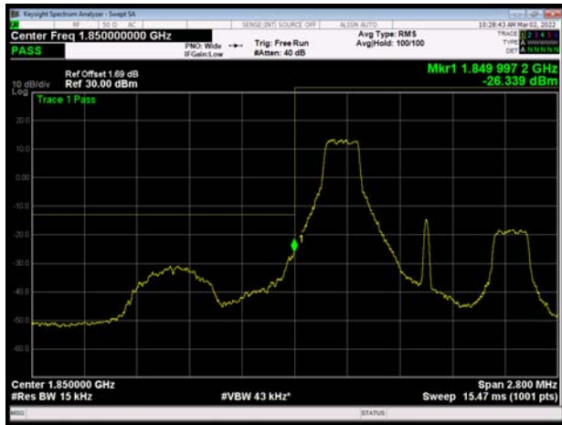
LTE Band 2 1.4MHz 16QAM 100%RB CH-Low
