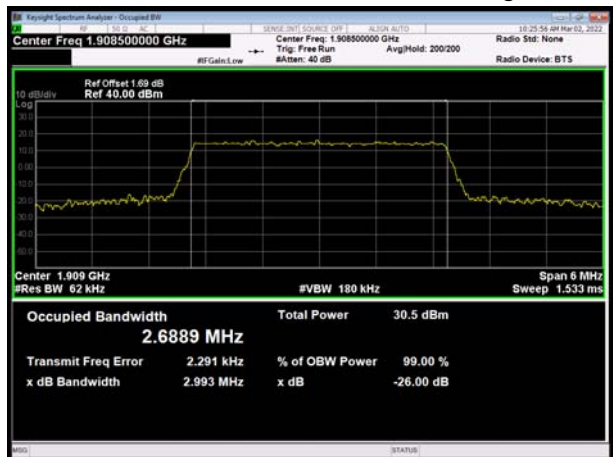
LTE Band 2 3MHz 16QAM CH-High
