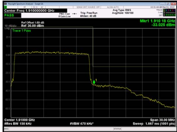
LTE Band 2 20MHz 16QAM 1RB CH-High
