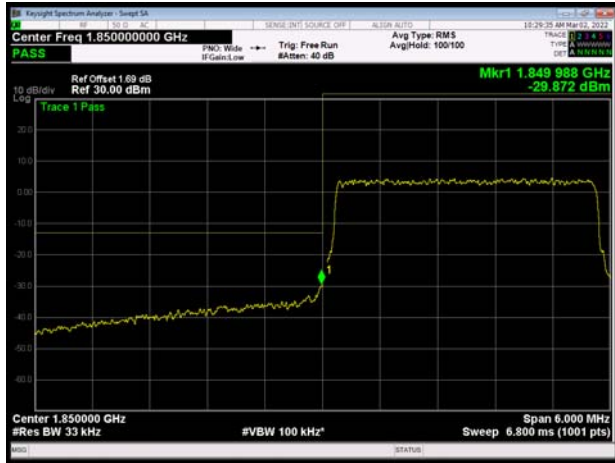
LTE Band 2 5MHz 16QAM 1RB CH-Low
