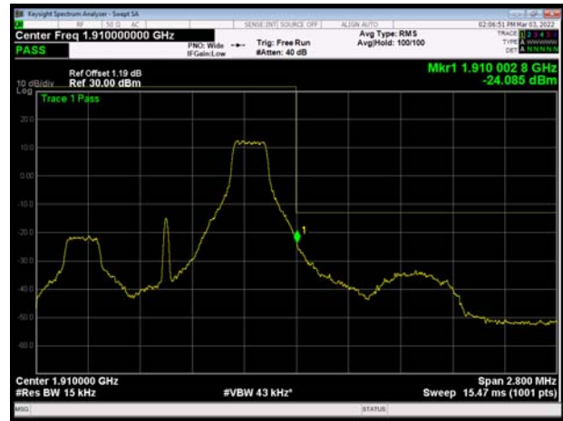
LTE Band 2 1.4MHz 64QAM 100%RB CH-High
