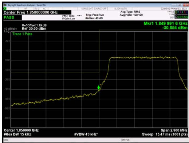
LTE Band 2 3MHz 64QAM 1RB CH-Low
