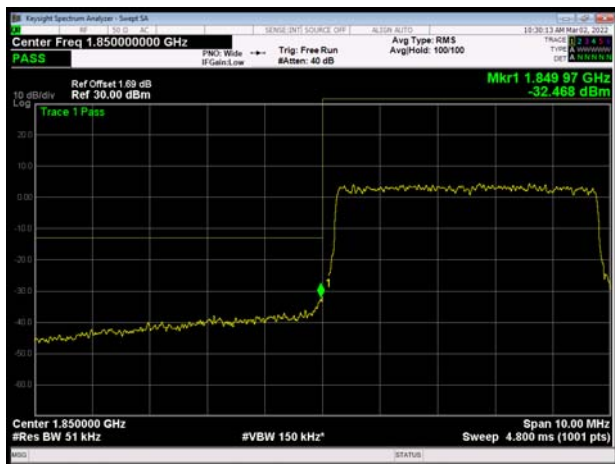
LTE Band 2 5MHz 16QAM 100%RB CH-Low
