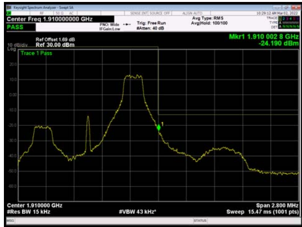
LTE Band 2 1.4MHz 16QAM 100%RB CH-High
