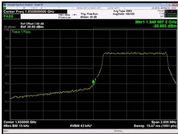
LTE Band 2 3MHz 16QAM 1RB CH-Low
