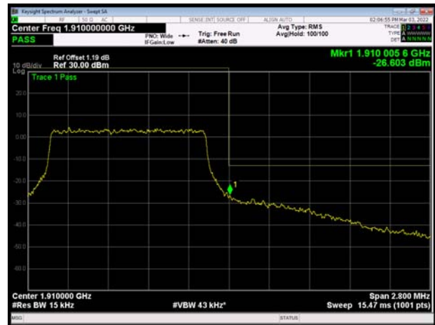
LTE Band 2 3MHz 64QAM 1RB CH-High
