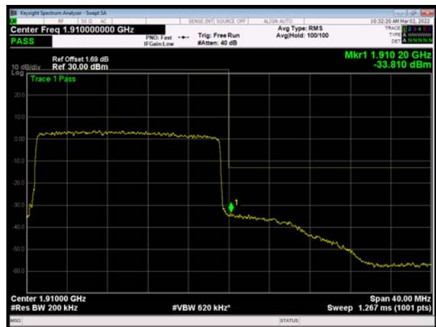
LTE Band 2 20MHz 16QAM 100%RB CH-High
