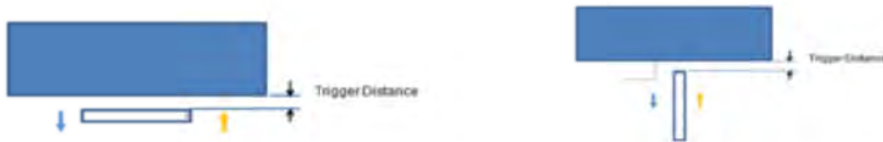
Picture : Proximity sensor triggering distances assessment(Back/front side)
