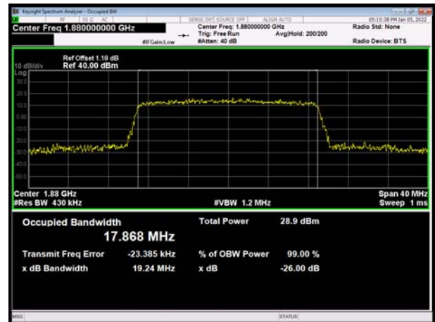
LTE Band 2 20MHz 64QAM CH-High
