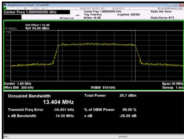
LTE Band 2 15MHz 64QAM CH-High
