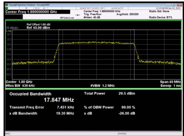
LTE Band 2 20MHz 16QAM CH-High
