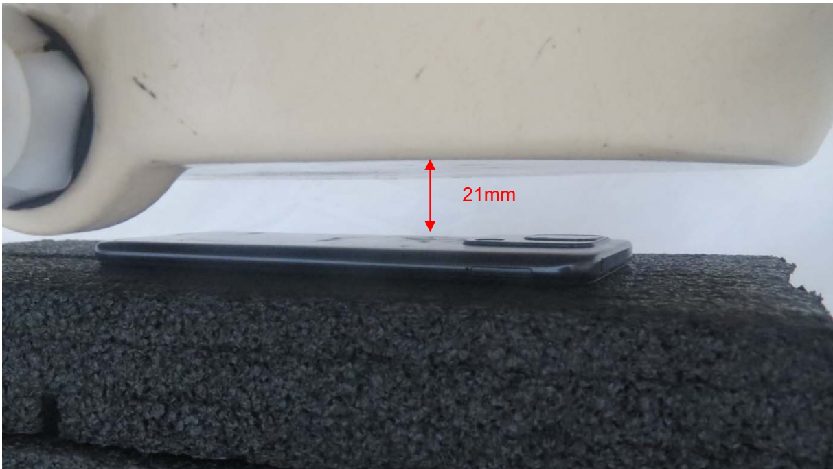
Picture 17: Back Side, the distance from handset to the bottom of the Phantom is 21mm
