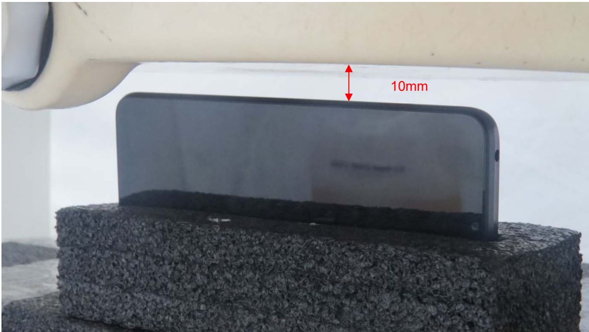
Picture 7: Left Side, the distance from handset to the bottom of the Phantom is 10mm
