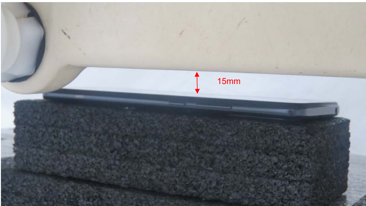
Picture 18: Front Side, the distance from handset to the bottom of the Phantom is 15mm
