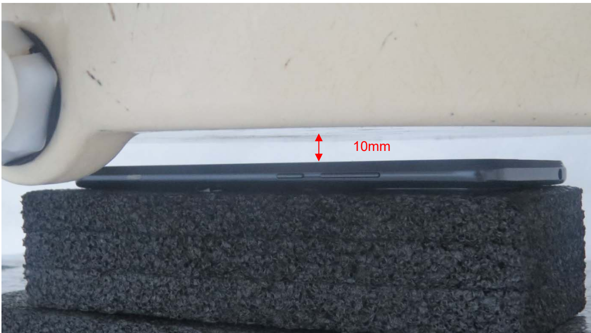
Picture 6: Front Side, the distance from handset to the bottom of the Phantom is 10mm
