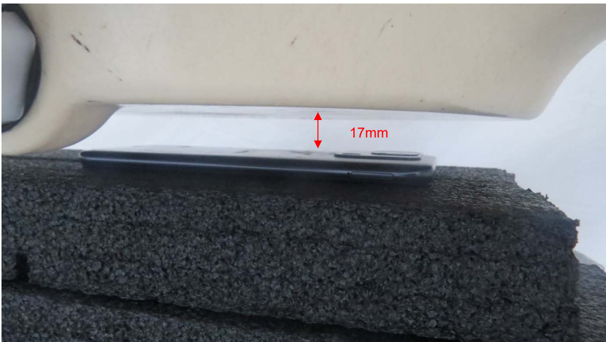
Picture 16: Back Side, the distance from handset to the bottom of the Phantom is 17mm
