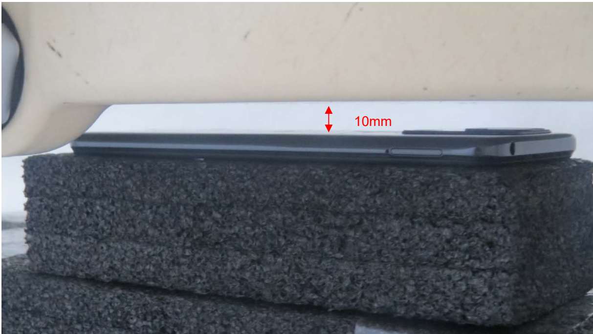
Picture 5: Back Side, the distance from handset to the bottom of the Phantom is 10mm
