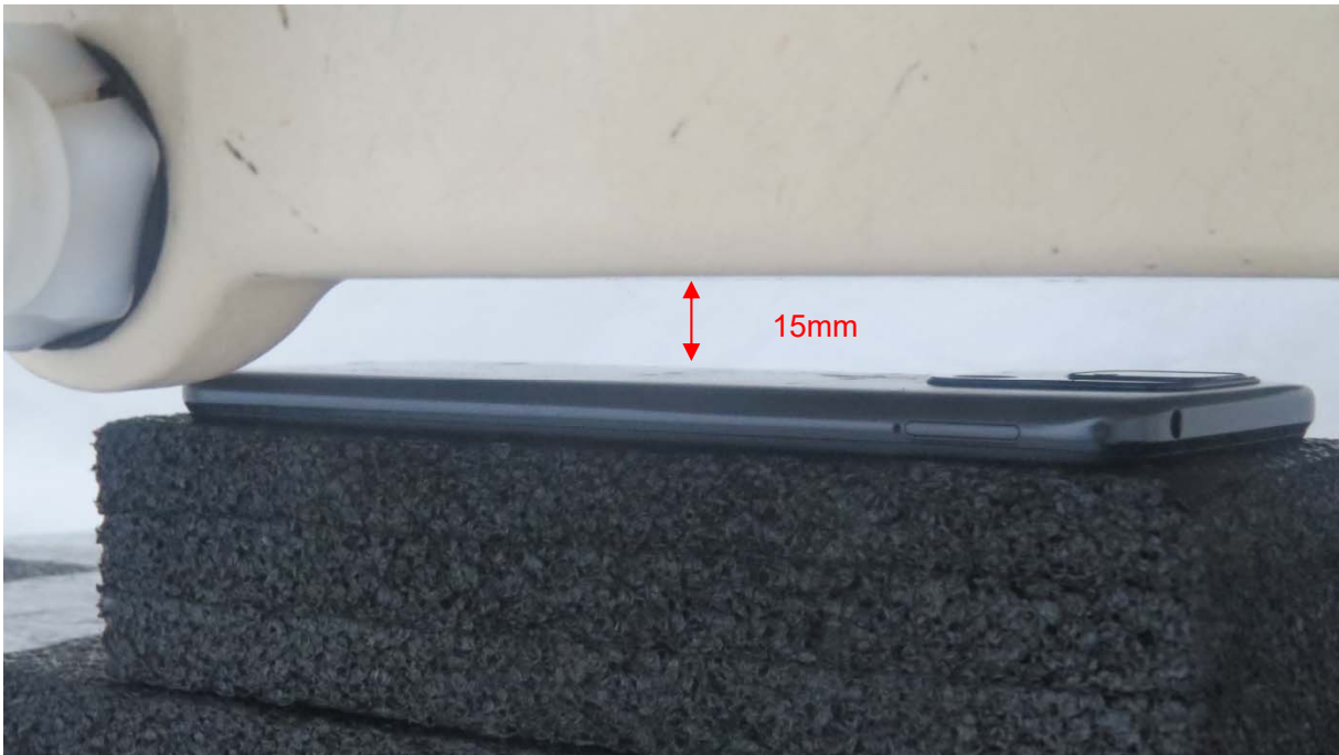
Picture 15: Back Side, the distance from handset to the bottom of the Phantom is 15mm
