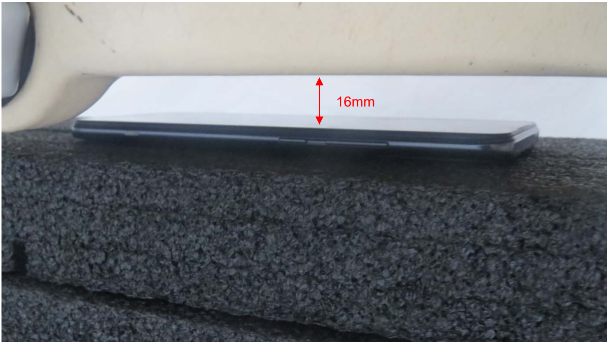
Picture 19: Front Side, the distance from handset to the bottom of the Phantom is 16mm
