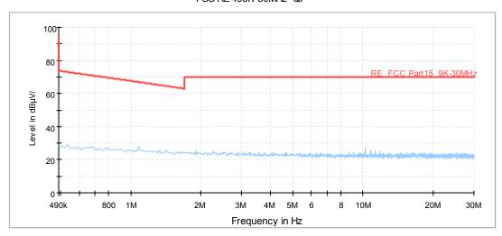
Radiates Emission from 490KHz to 30MHz
