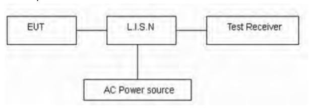
Note: AC Power source is used to change the voltage 110V/60Hz.
