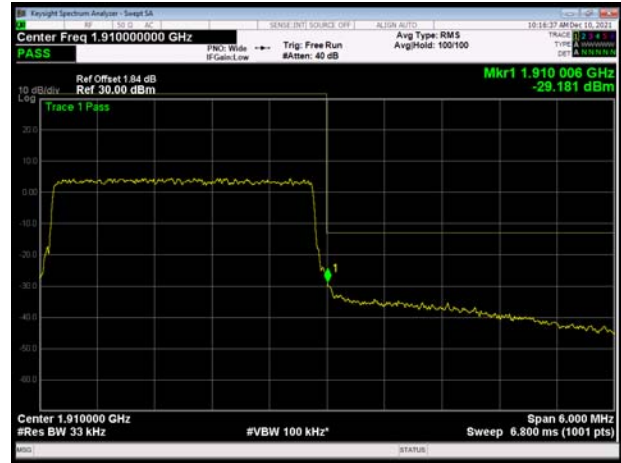
LTE Band 2 5MHz QPSK 1RB CH-High
