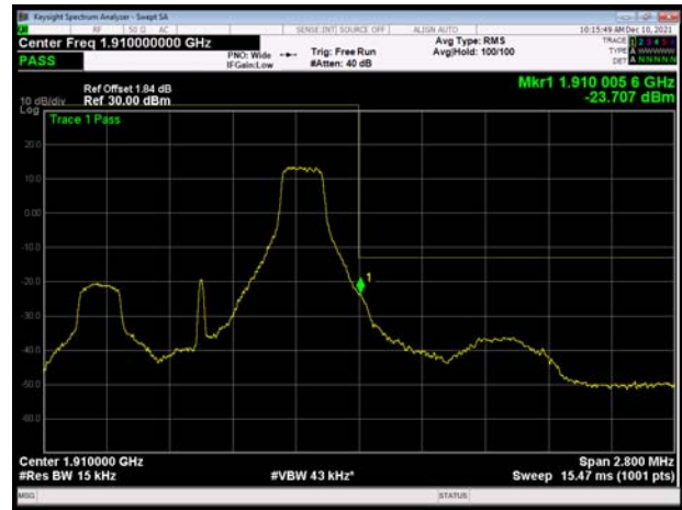
LTE Band 2 1.4MHz QPSK 100%RB CH-High
