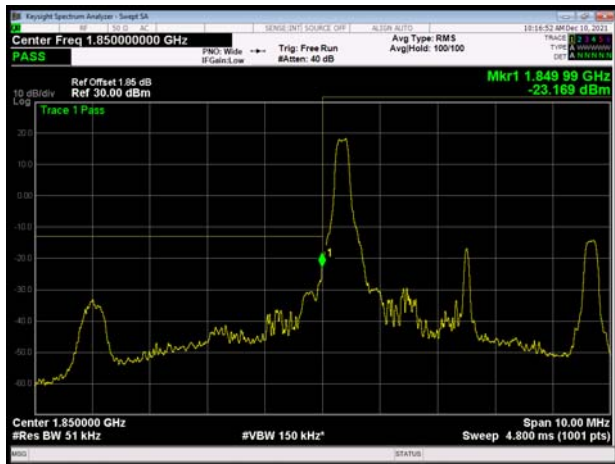
LTE Band 2 5MHz QPSK 100%RB CH-Low
