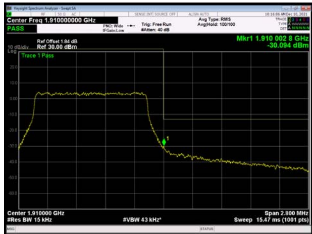
LTE Band 2 3MHz 16QAM 1RB CH-High
