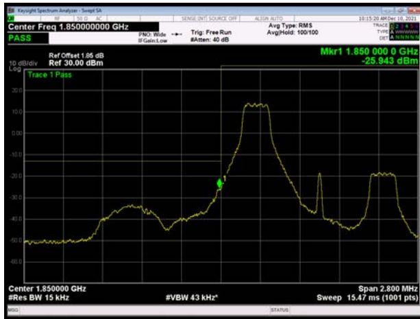
LTE Band 2 1.4MHz QPSK 100%RB CH-Low
