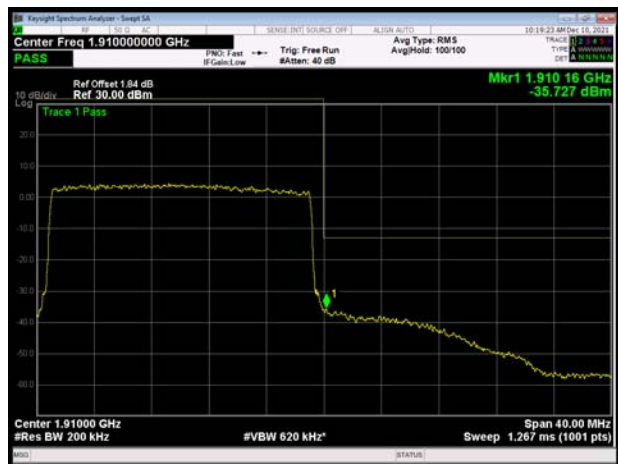
LTE Band 2 20MHz QPSK 100%RB CH-High
