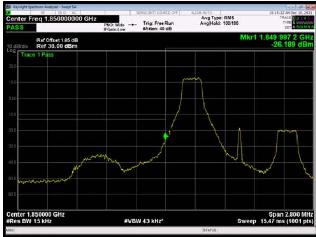
LTE Band 2 1.4MHz 16QAM 100%RB CH-Low
