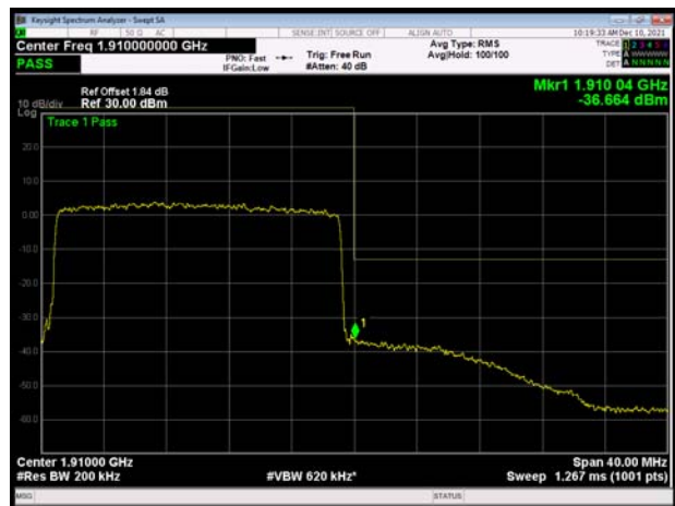
LTE Band 2 20MHz 16QAM 100%RB CH-High
