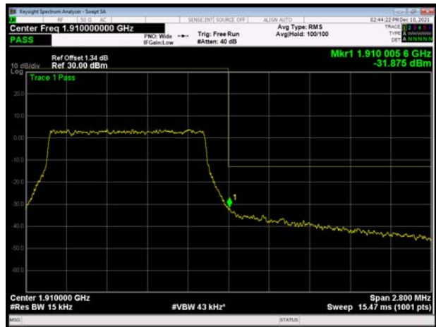
LTE Band 2 3MHz 64QAM 1RB CH-High
