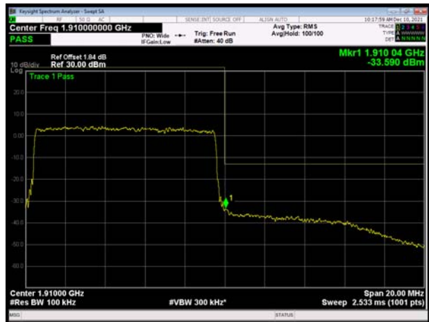
LTE Band 2 15MHz QPSK 1RB CH-High
