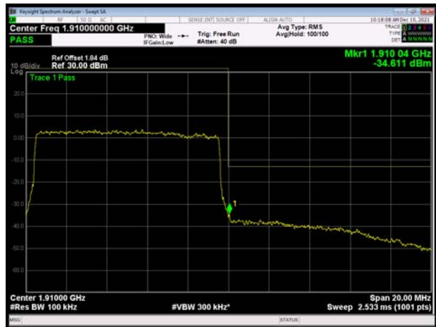
LTE Band 2 15MHz 16QAM 1RB CH-High
