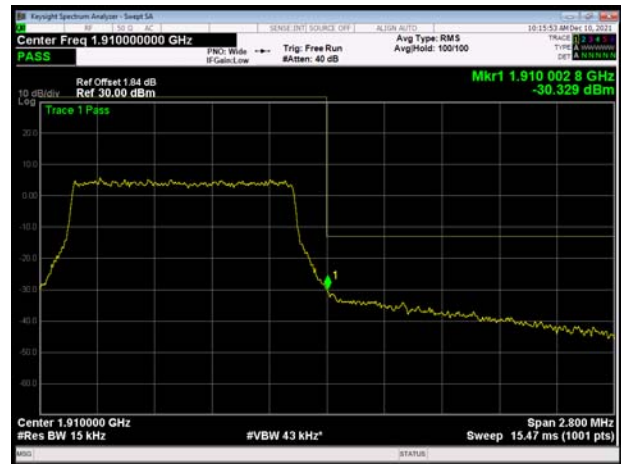
LTE Band 2 3MHz QPSK 1RB CH-High
