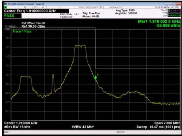
LTE Band 2 1.4MHz 16QAM 100%RB CH-High
