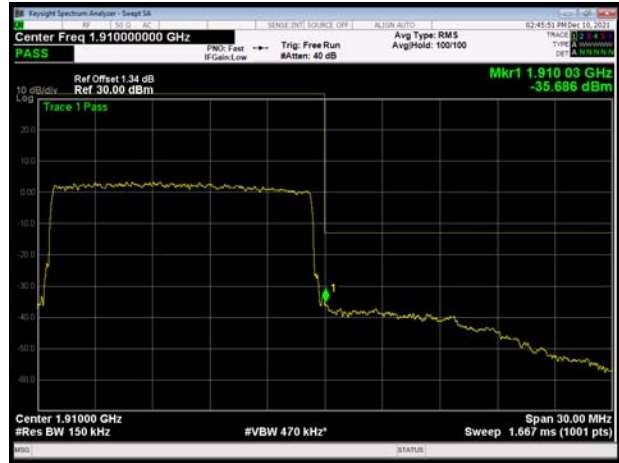
LTE Band 2 20MHz 64QAM 1RB CH-High
