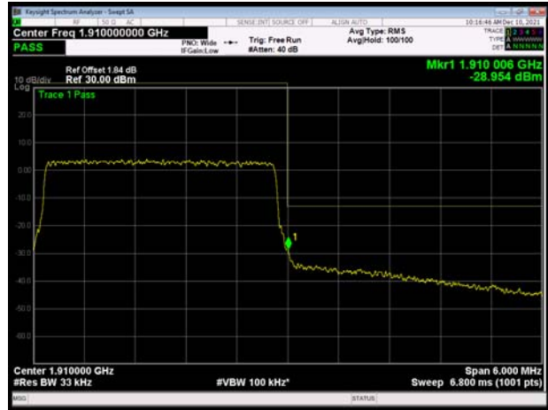
LTE Band 2 5MHz 16QAM 1RB CH-High
