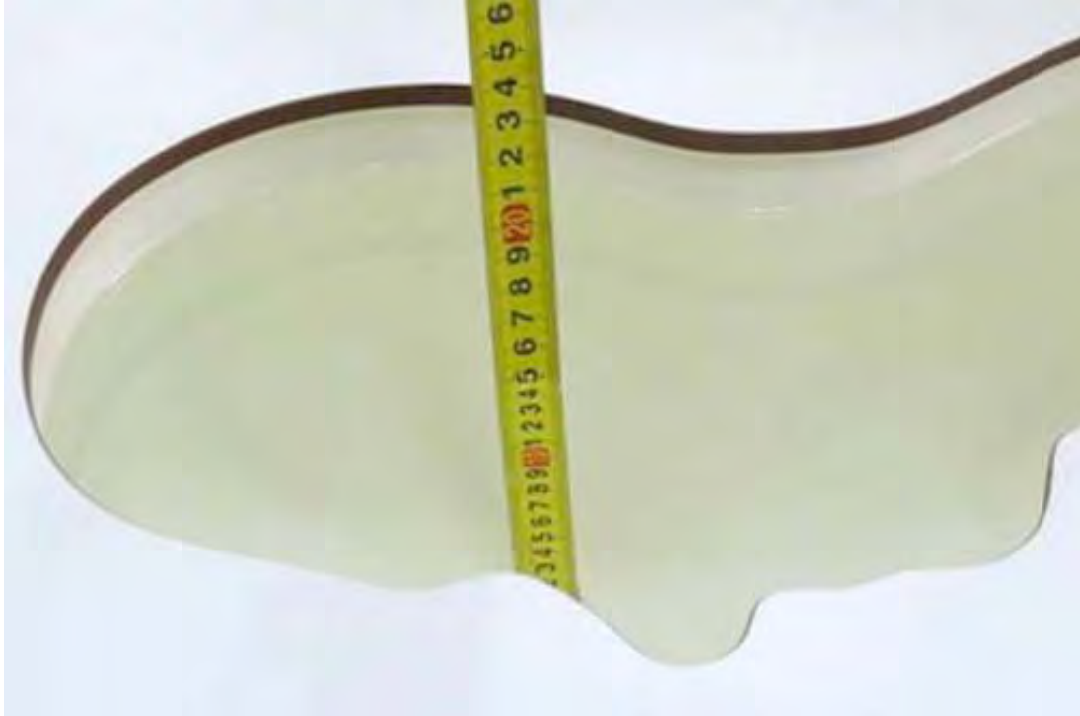
Picture 3: liquid depth in the head Phantom
