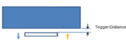
Picture : Proximity sensor triggering distances assessment(Back/front side)
