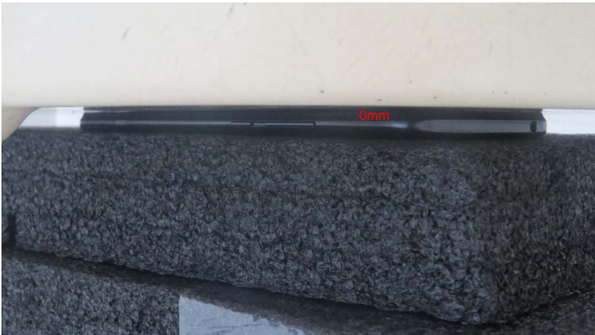
Picture 12: Front Side, the distance from handset to the bottom of the Phantom is 0mm
