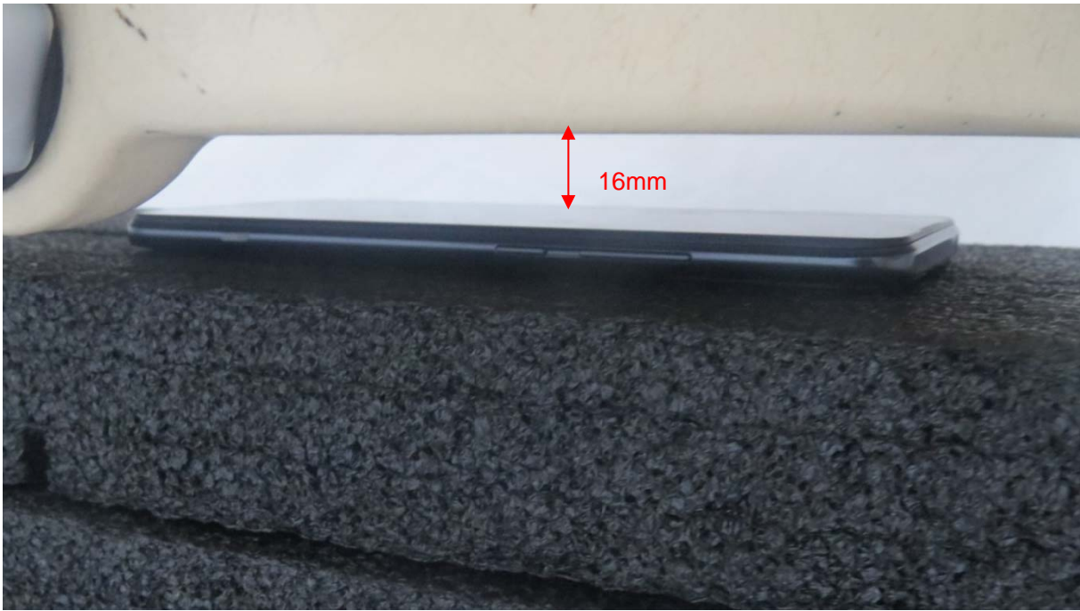
Picture 17: Front Side, the distance from handset to the bottom of the Phantom is 16mm
