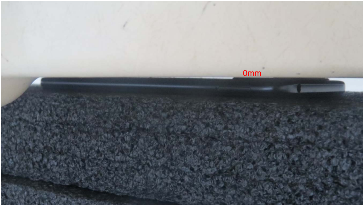
Picture 11: Back Side, the distance from handset to the bottom of the Phantom is 0mm
