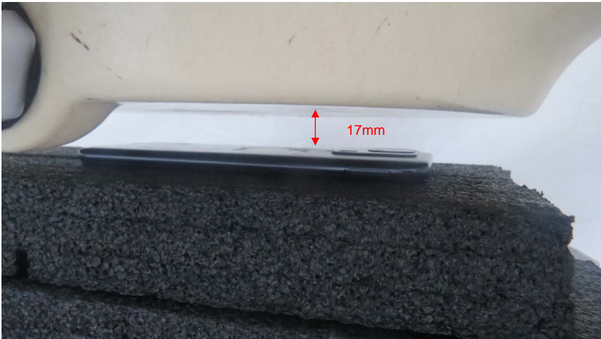
Picture 15: Back Side, the distance from handset to the bottom of the Phantom is 17mm
