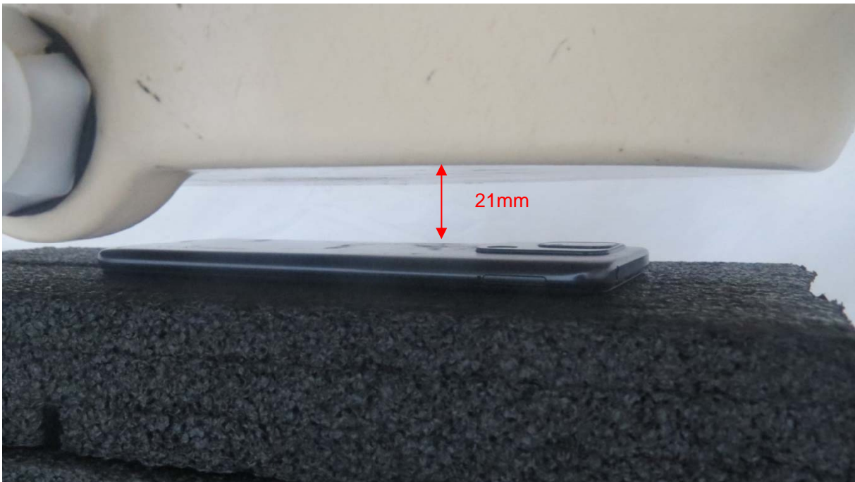
Picture 16: Back Side, the distance from handset to the bottom of the Phantom is 21mm
