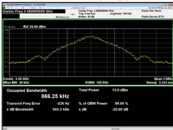
BT DH5 CH78, Carrier frequency (MHz): 2480
