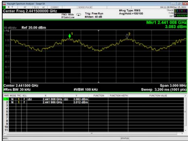
BT DH5 CH78, Carrier frequency (MHz): 2480
