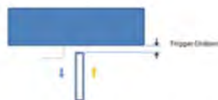
Picture : Proximity sensor triggering distances assessment(Top/Bottom edge)
