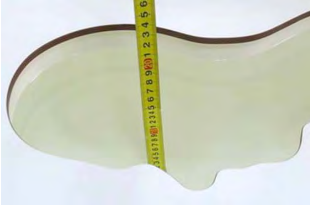
Picture 3: liquid depth in the head Phantom
