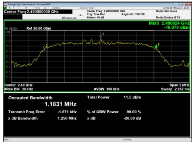
BT 2DH5 CH78, Carrier frequency (MHz): 2480
