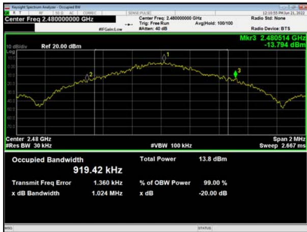
BT DH5 CH78, Carrier frequency (MHz): 2480
