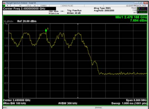
BT DH5 CH78, Carrier frequency (MHz): 2480
