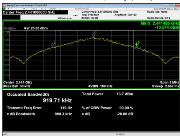
BT DH5 CH78, Carrier frequency (MHz): 2480
