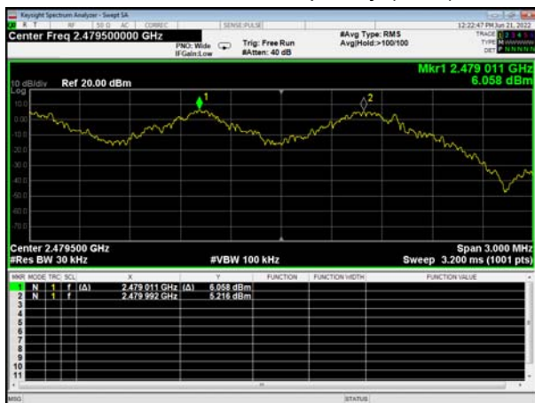
BT DH5 CH78, Carrier frequency (MHz): 2480
