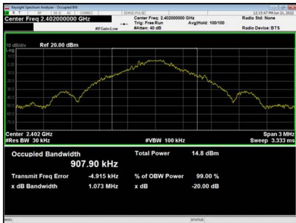
BT DH5 CH39, Carrier frequency (MHz): 2441
