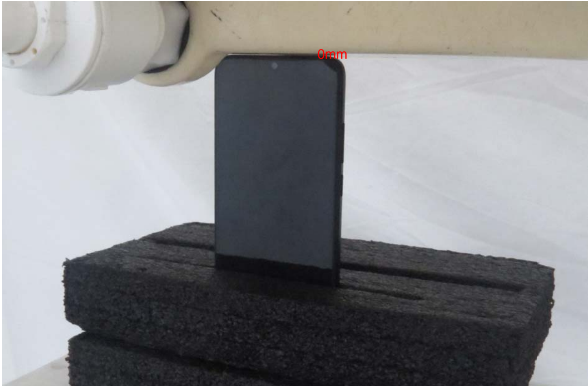
Picture 17: Top Edge, the distance from handset to the bottom of the Phantom is 0mm
