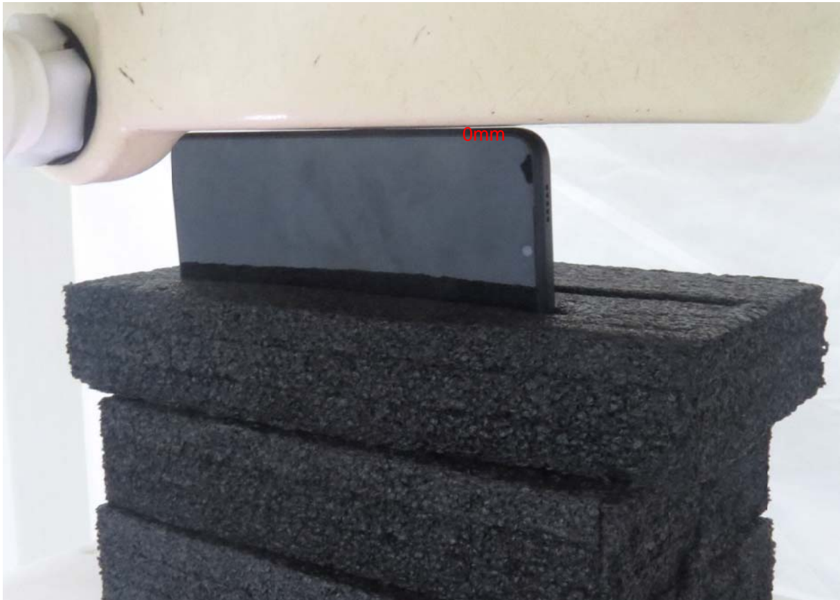
Picture 15: Left Edge, the distance from handset to the bottom of the Phantom is 0mm
