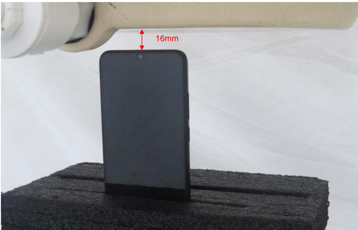
Picture 20: Top Edge, the distance from handset to the bottom of the Phantom is 16mm
