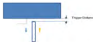
Picture : Proximity sensor triggering distances assessment(Top/Bottom edge)
