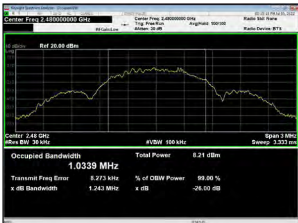
Bluetooth LE (1M) Carrier frequency (MHz): 2480
