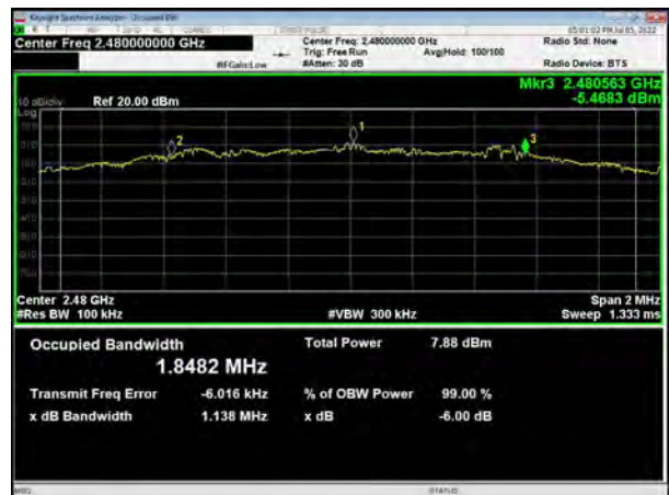
Bluetooth LE (2M) Carrier frequency (MHz): 2480
