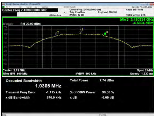
Bluetooth LE (1M) Carrier frequency (MHz): 2480
