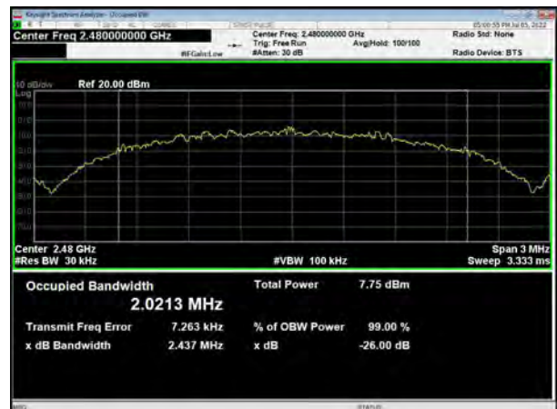
Bluetooth LE (2M) Carrier frequency (MHz): 2480
