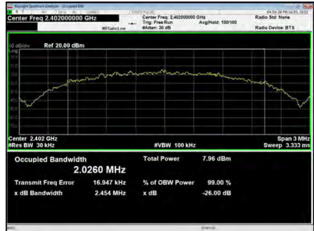
Bluetooth LE (2M) Carrier frequency (MHz): 2440
