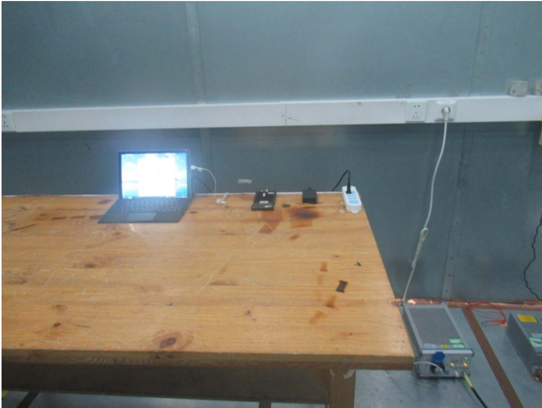
Picture 2: Conducted Emissions Test Setup
