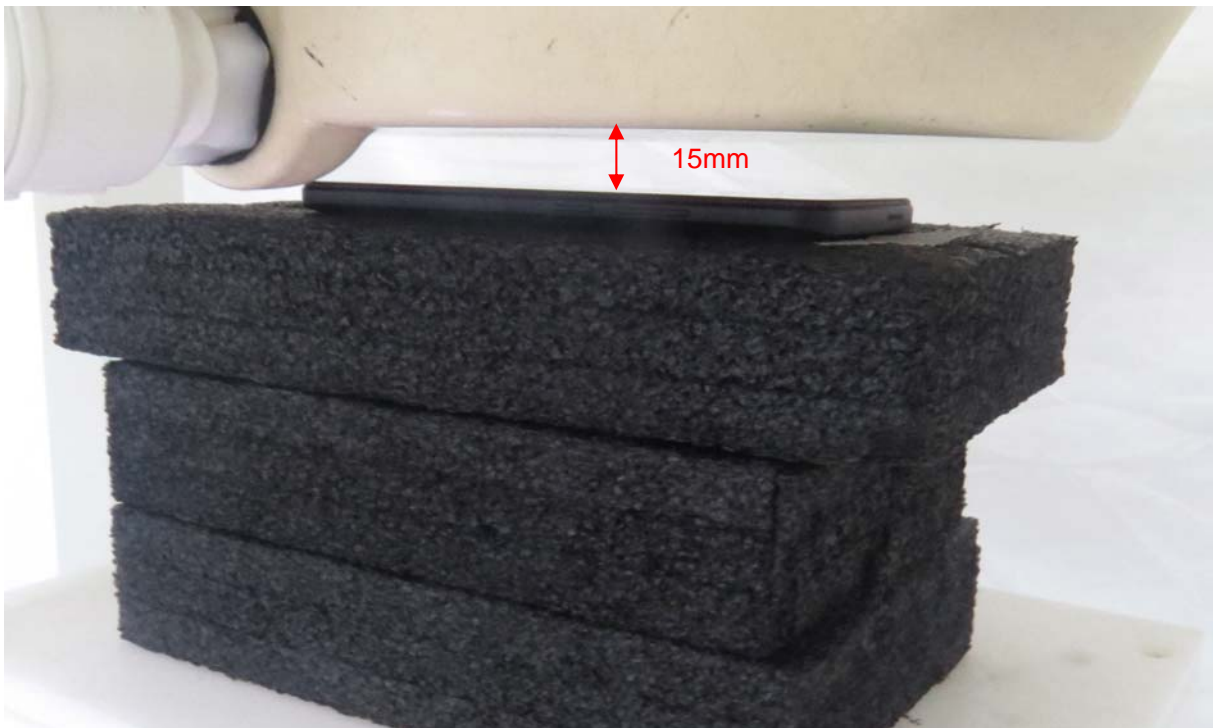
Picture 6: Front Side, the distance from handset to the bottom of the Phantom is 15mm
