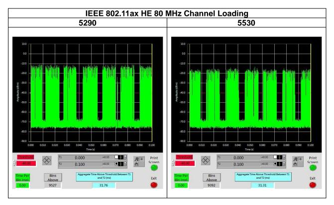
Note: During the monitoring period of 100ms, the packet flow exceeds 17%
