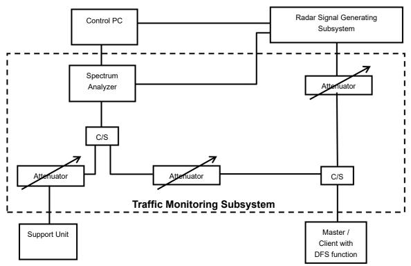
The test transmission will always be from the Master Device to the Client Device. While the Client device is set up to associate with the Master device and play the MPEG file (6  $\psi$  Magic Hours) from Master device, the designated MPEG test file and instructions are located at: <a href="http://ntiacsd.ntia.doc.gov/dfs/">http://ntiacsd.ntia.doc.gov/dfs/</a>.
