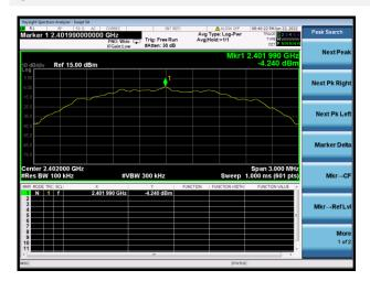
GFSK (BLE 2Mbps) LOW CHANNEL, SPURIOUS 30 MHz ~ 3 GHz
