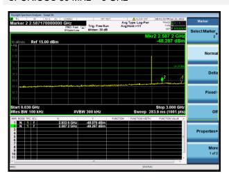
GFSK (BLE 2Mbps) LOW CHANNEL, SPURIOUS 2 GHz ~ 25 GHz
