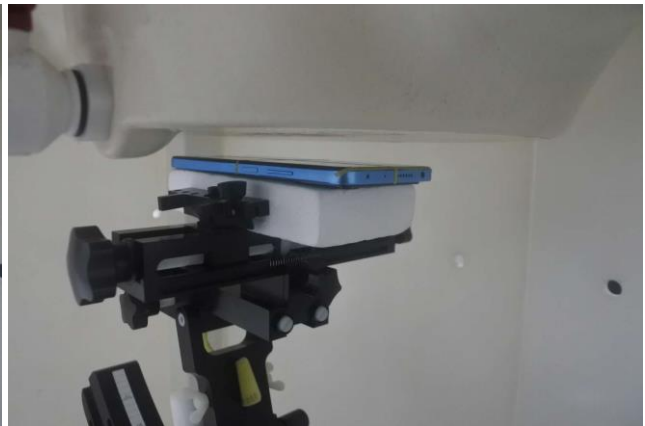
Back, Test Separation 15 mm(sensor off)
