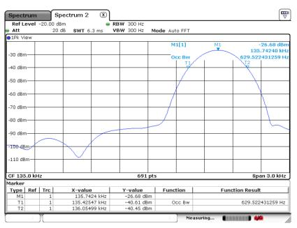
**Remark:** Because the measured signal is CW adjusting the RBW per C63.10 would not be practical since measured bandwidth will always follow the RBW and the result will be approximately twice the RBW.
