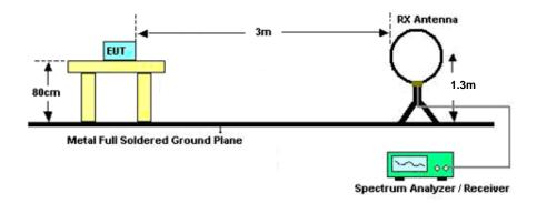
**Note:** There is a comparison data of both open-field test site and alternative test site - semi-Anechoic chamber according to 414788 D01 Radiated Test Site v01r01, and the result came out very similar. **For radiated emissions above 30MHz**
