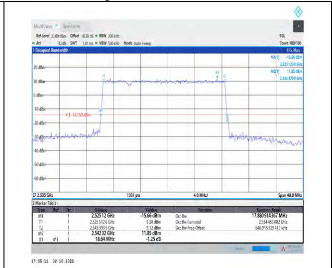
1-N7--15-20-M-4-DFT-64QAM-Outer_Full-100@0-An t1-17.881-18.640- \leq 20 -PASS
