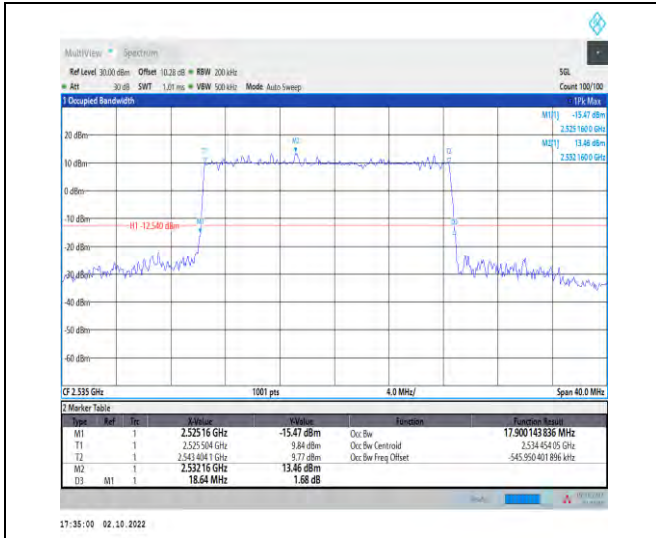
1-N7--15-20-M-3-DFT-16QAM-Outer_Full-100@0-An t1-17.9-18.640- \leq 20 -PASS
