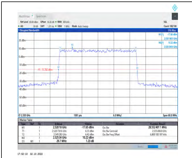
1-N7--15-30-M-5-DFT-256QAM-Outer_Full-160@0-A nt1-28.552-29.700- \leq 30 -PASS
