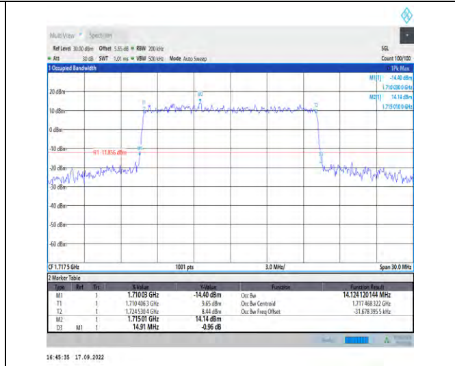
1-N66--15-15-L-8-CP-64QAM-Outer_Full-79@0-Ant 1-14.124-14.910≤15-PASS
