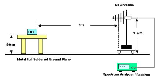
For radiated test from 1GHz to 18GHz
