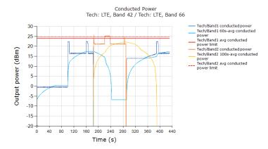
Plot Notes: ... The conducted power plot shows expected transitions in Tx power at ~185 seconds (60s-to-100s transition) and at ~290 seconds (100s-to-60s transition) in order to maintain total time-averaged RF exposure compliance across time windows, as show in next plot.
