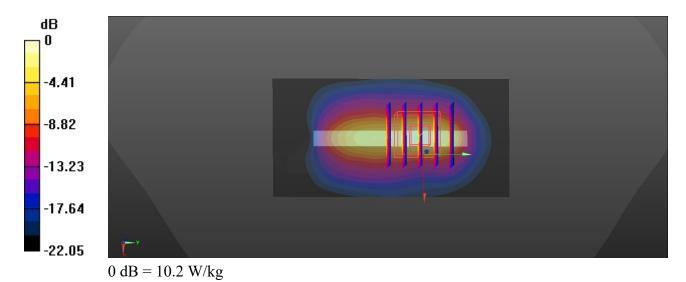
Communication System: UID 0, LTE (0); Frequency: 2535 MHz; Duty Cycle: 1:1
