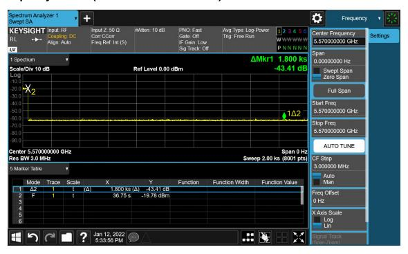
**Verdict:** To verify whether channel is unavailable to be operated in 30 minutes. 1.8ks = 1800s = 1800 s/min / 60 = 30 minute
