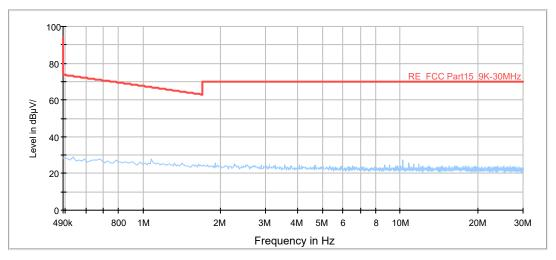
Radiates Emission from 490KHz to 30MHz
