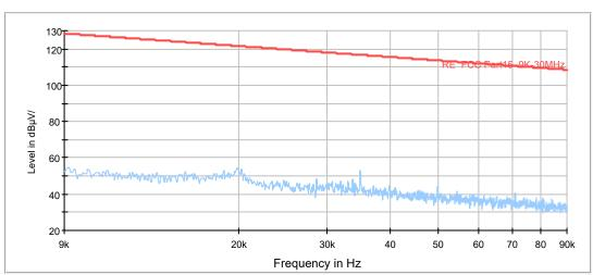
Radiates Emission from 9KHz to 90KHz
