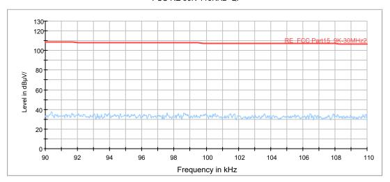
Radiates Emission from 90KHz to 110KHz
