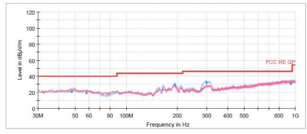
Radiates Emission from 30MHz to 1GHz Note: This graph displays the maximum values of horizontal and vertical by software
