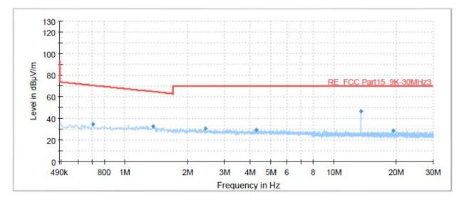
Radiates Emission from 490kHz to 30MHz
