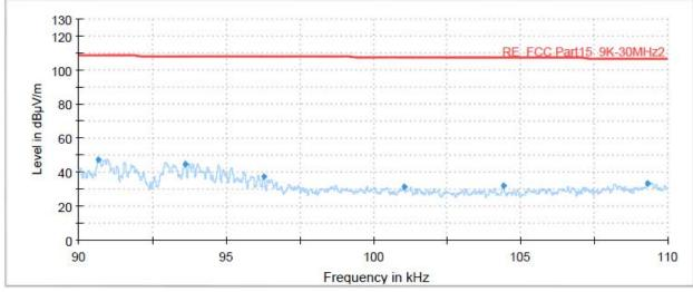
Radiates Emission from 90kHz to 110kHz
