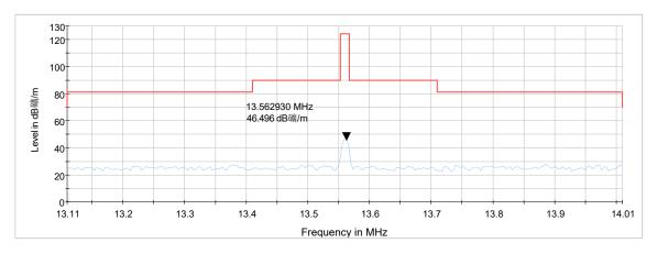
Radiates Emission from 13.11MHz to 14.01MHz Note: This graph displays the maximum values of horizontal and vertical by software
