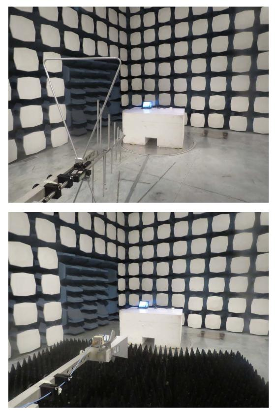
Picture 1: Radiated Emission Test Setup
