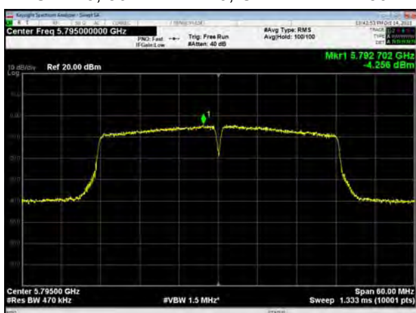
U-NII-3, 802.11ac VHT40, Channel No.: 151
