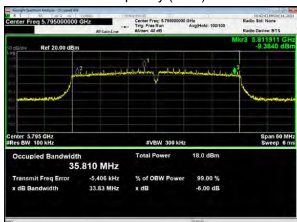
U-NII-3, 802.11n HT40 Carrier frequency (MHz): 5795
