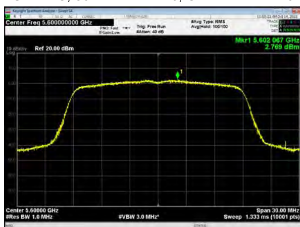
U-NII-2C, 802.11ac VHT20, Channel No.: 140
