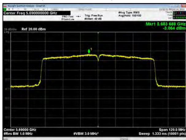
U-NII-2C, 802.11ac VHT80, Channel No.: 138
