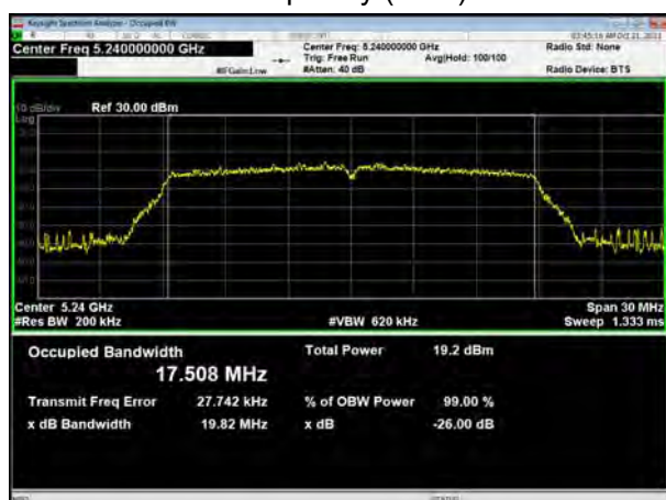
U-NII-1, 802.11n HT20 Carrier frequency (MHz): 5240
