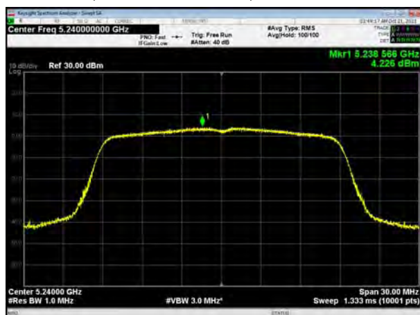
U-NII-1, 802.11ac VHT20, Channel No.: 48
