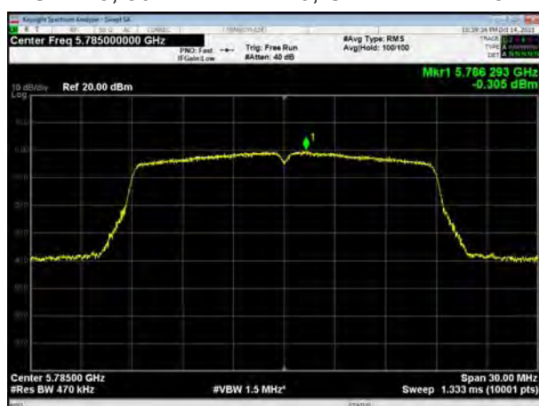
U-NII-3, 802.11ac VHT20, Channel No.: 165
