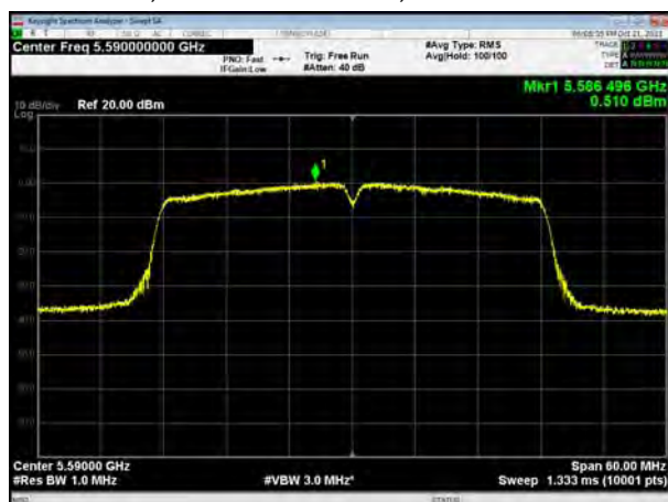
U-NII-2C, 802.11ac VHT40, Channel No.: 144
