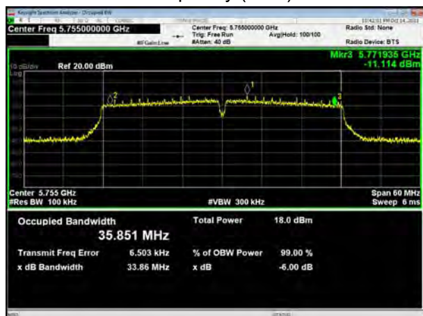
U-NII-3, 802.11n HT40 Carrier frequency (MHz): 5795
