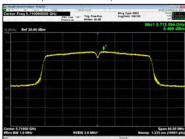
U-NII-2C, 802.11ac VHT80, Channel No.: 138
