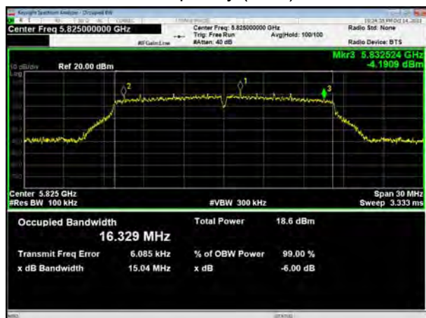
U-NII-3, 802.11n HT40 Carrier frequency (MHz): 5755
