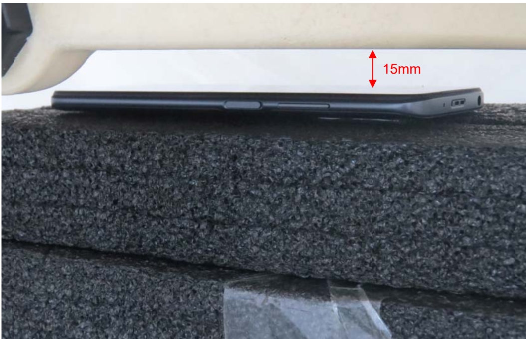
Picture 6: Front Side, the distance from handset to the bottom of the Phantom is 15mm
