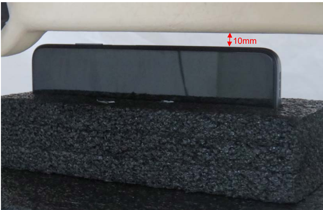
Picture 12: Right Edge, the distance from handset to the bottom of the Phantom is 10mm
