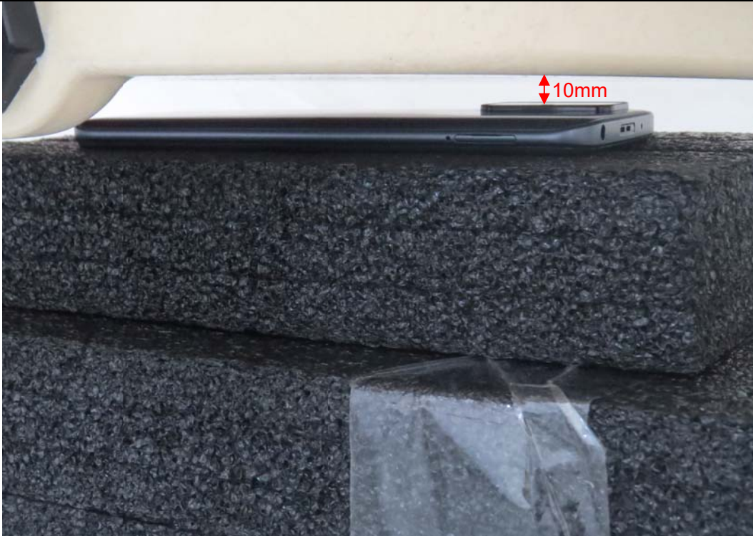
Picture 9: Back Side, the distance from handset to the bottom of the Phantom is 10mm
