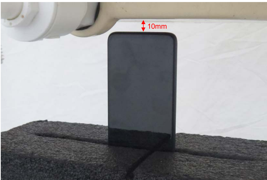
Picture 14: Bottom Edge, the distance from handset to the bottom of the Phantom is 10mm
