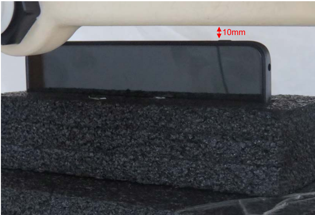
Picture 11: Left Edge, the distance from handset to the bottom of the Phantom is 10mm
