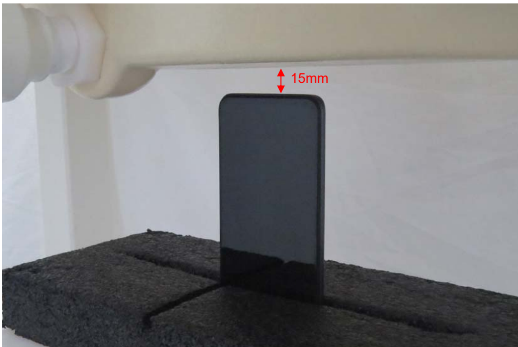
Picture 8: Bottom Edge, the distance from handset to the bottom of the Phantom is 15mm
