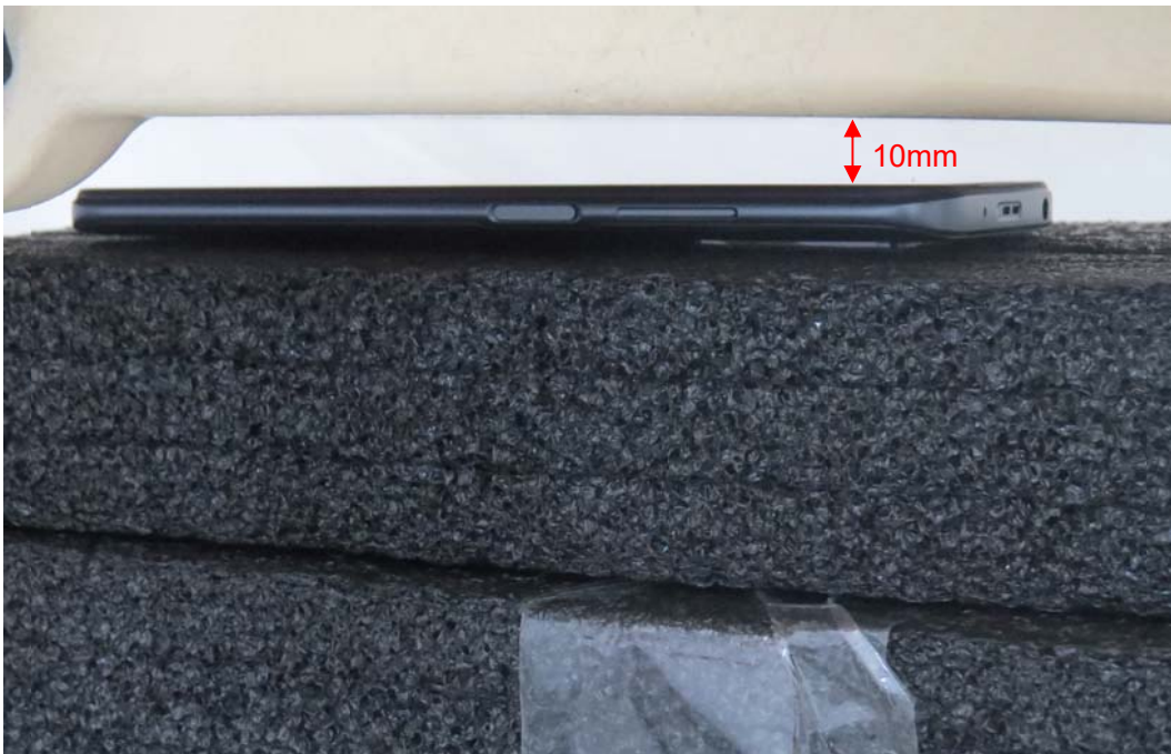
Picture 10: Front Side, the distance from handset to the bottom of the Phantom is 10mm
