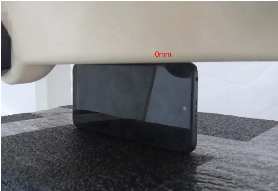
Picture 17: Left Edge, the distance from handset to the bottom of the Phantom is 0mm
