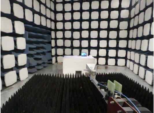
**Picture 1: Radiated Emission Test Setup**
