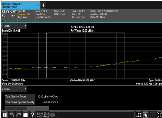
N66(40M)_DFT-s- OFDM_QPSK_Edge_1RB_Left_Low_CH_chp PASS
