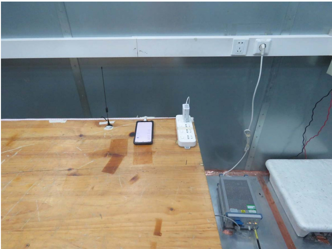
Picture 2 Conducted Emission Test Setup
