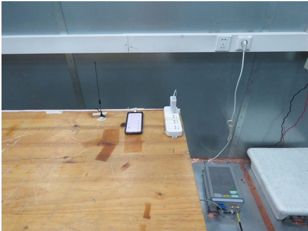
Picture 2 Conducted Emission Test Setup
