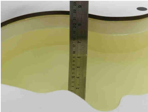
Fig 11.1 Photo of Liquid Height for Head SAR
