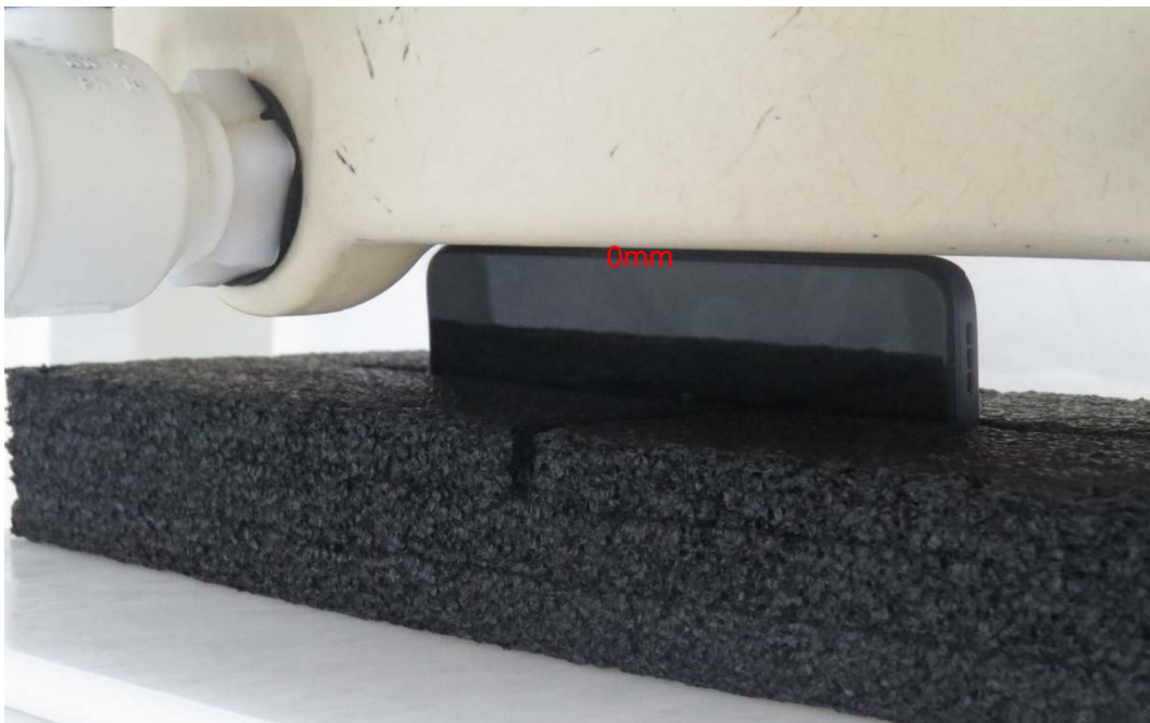
Picture 16: Right Side, the distance from handset to the bottom of the Phantom is 0mm
