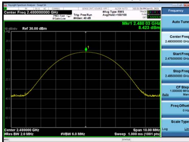
BT DH5 CH78, Carrier frequency (MHz): 2480
