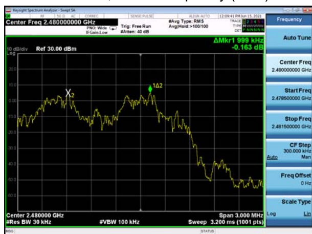
BT 2DH5 CH78, Carrier frequency (MHz): 2480
