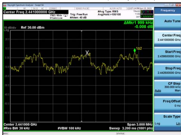
BT 2DH5 CH78, Carrier frequency (MHz): 2480
