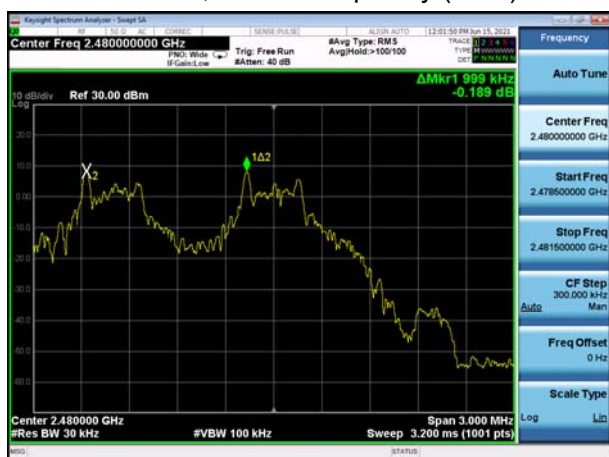
BT DH5 CH78, Carrier frequency (MHz): 2480
