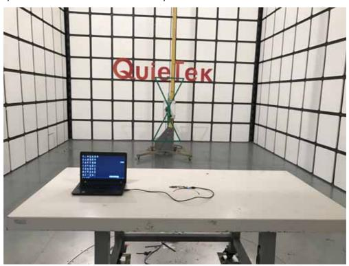
Description: Radiated Emission Test Setup for 1~18GHz
