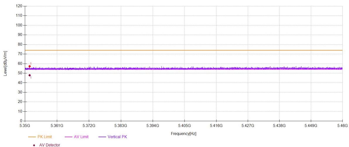
■ For Undesirable Radiated Spurious Emission in U-NII -2A
