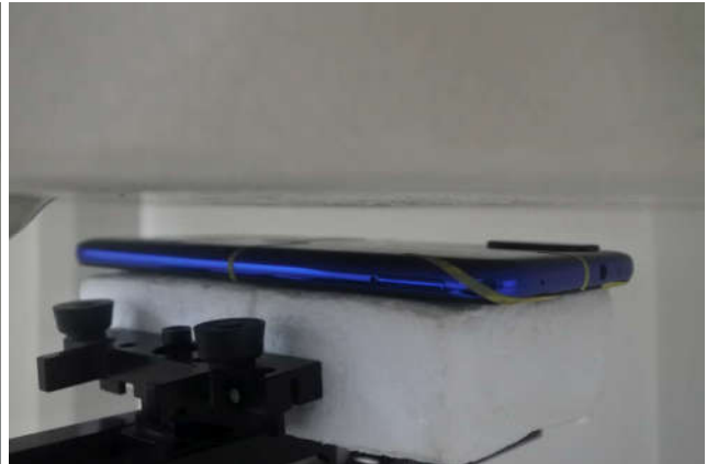
Back, Test Separation 10 mm
