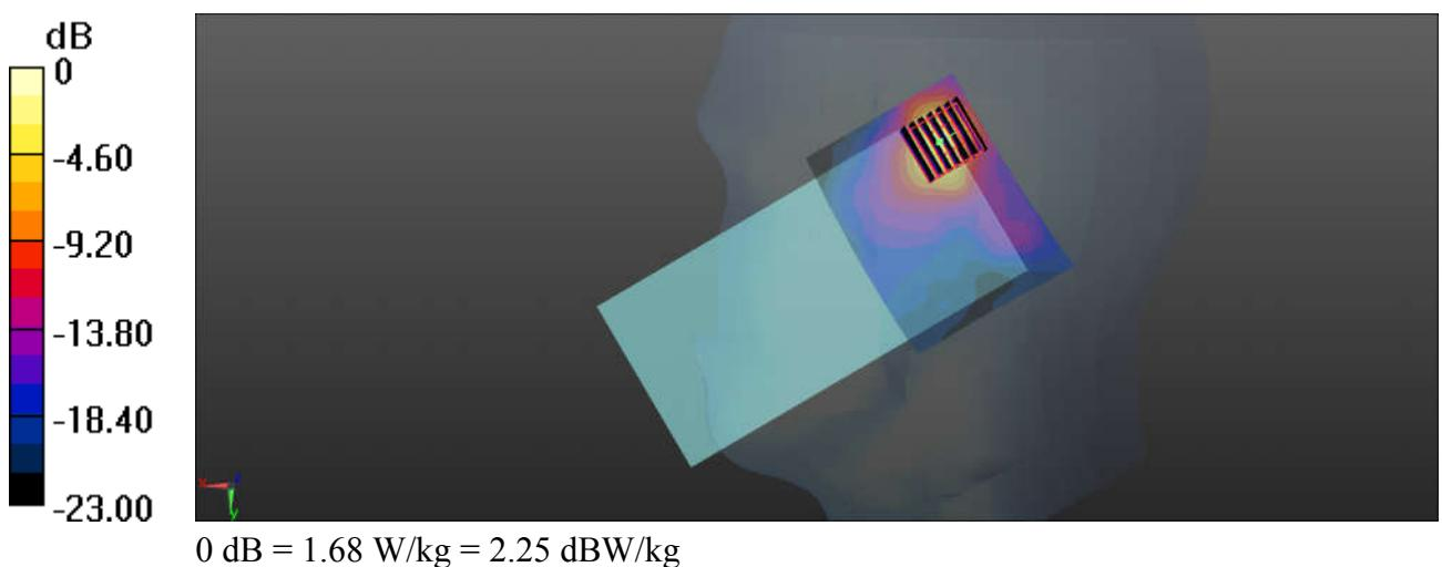
**20\_WLAN5.8GHz\_802.11a 6Mbps\_Right Cheek\_0mm\_Ant 2\_Ch149**
