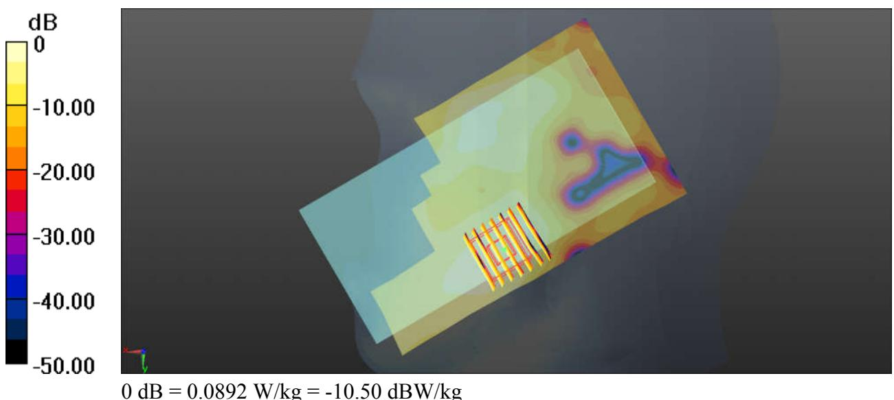
**13\_WLAN2.4GHz\_802.11b 1Mbps\_Right Cheek\_0mm\_Ant 1\_Ch11**
