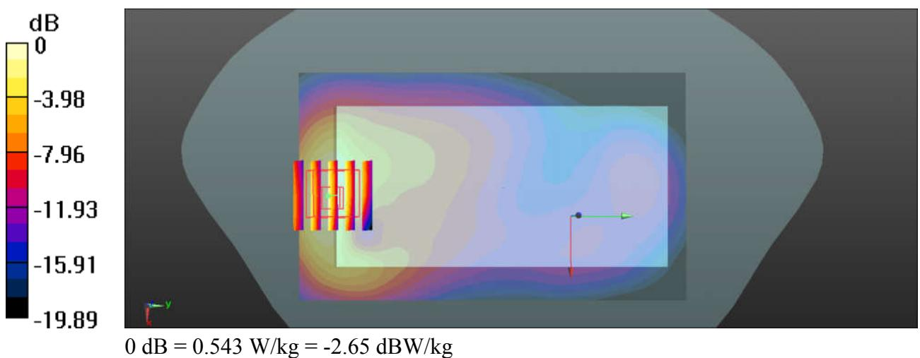
**50\_LTE Band 2\_20M\_QPSK\_1RB\_0Offset\_Back\_10mm\_Ch18900**
