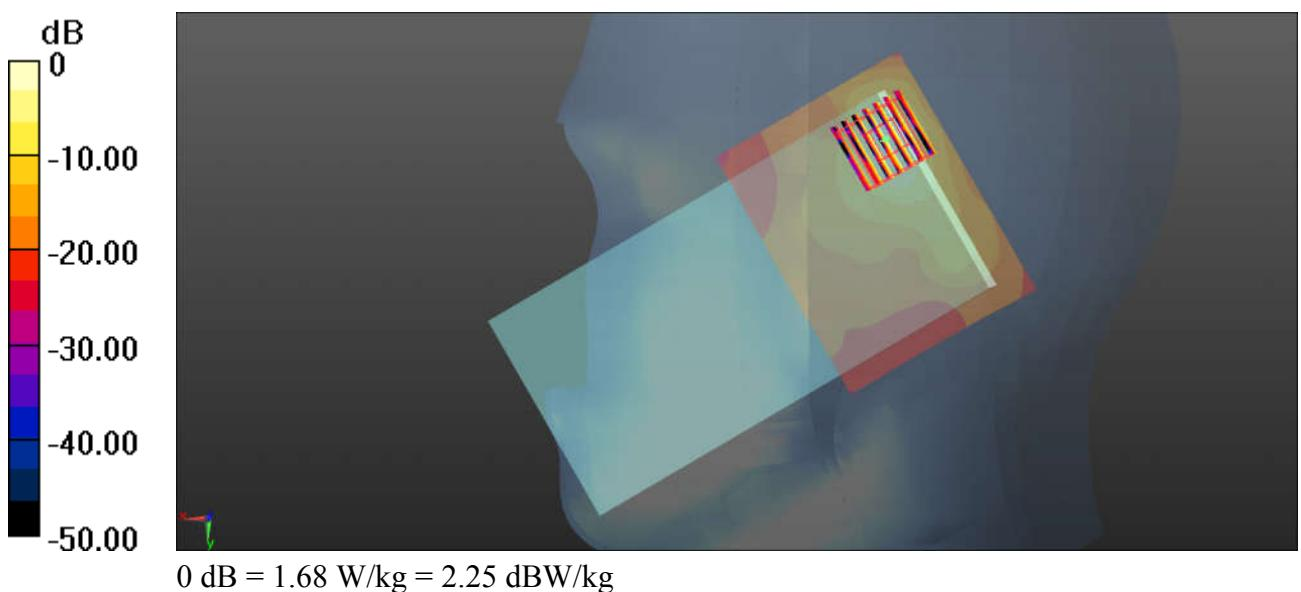
**18\_WLAN5.5GHz\_802.11a 6Mbps\_Right Cheek\_0mm\_Ant 2\_Ch100**
