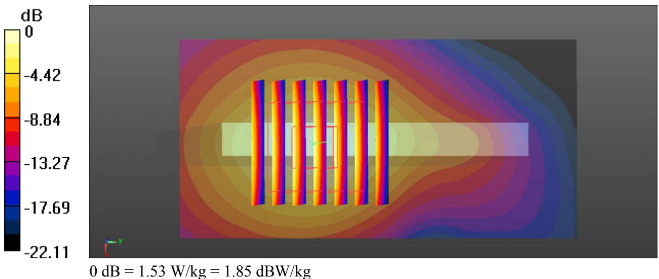
**33\_LTE Band 41\_20M\_QPSK\_1RB\_0Offset\_Bottom Side\_10mm\_Ch40400**
