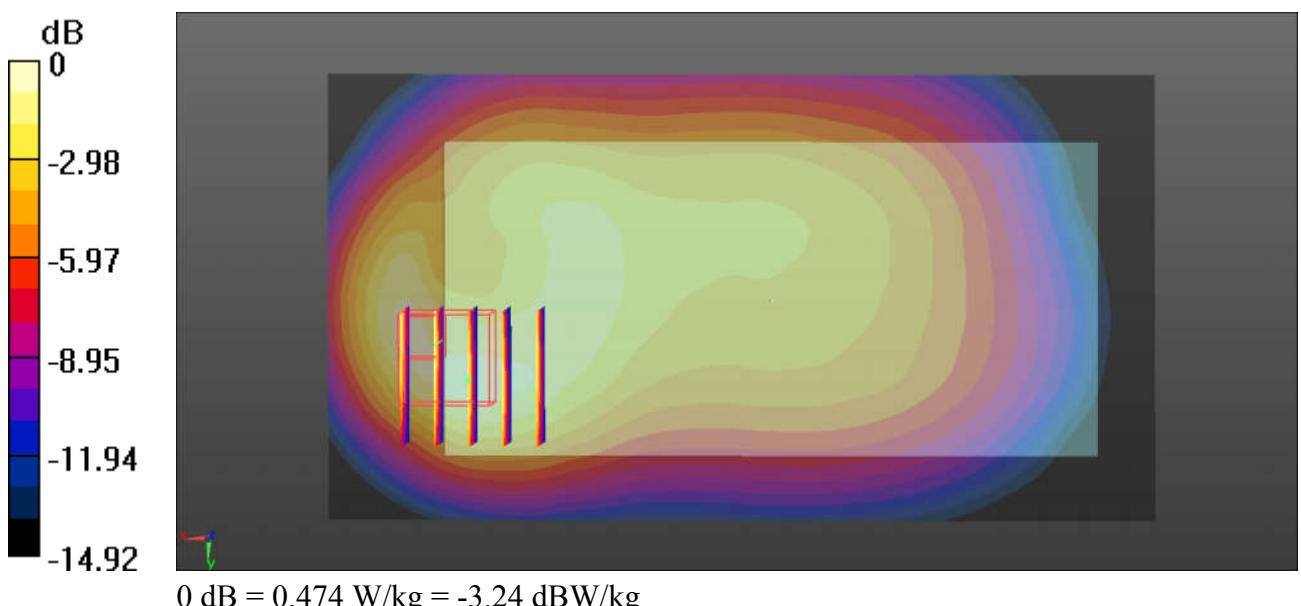
**49\_LTE Band 4\_20M\_QPSK\_1RB\_0Offset\_Back\_10mm\_Ch20175**
