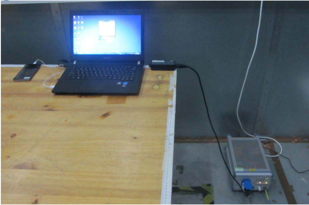
Conducted Emission Test Setup
