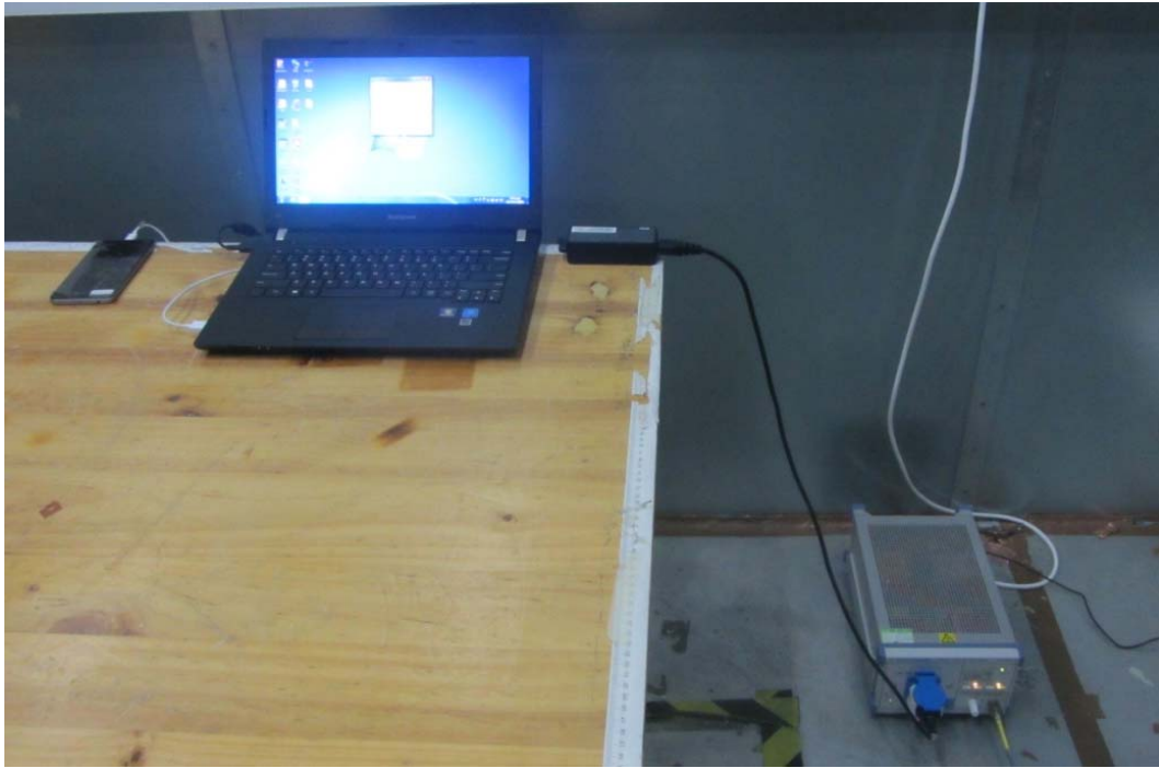
Picture 3 Conducted Emission Test Setup
