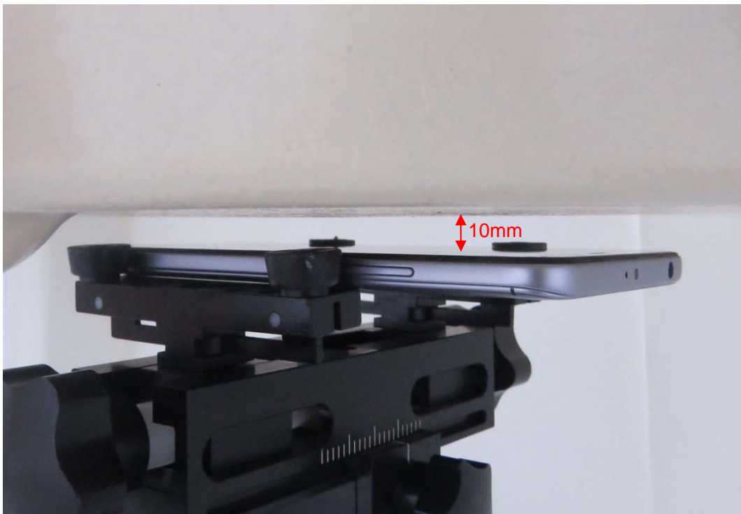
Front Side, the distance from handset to the bottom of the Phantom is 10mm
