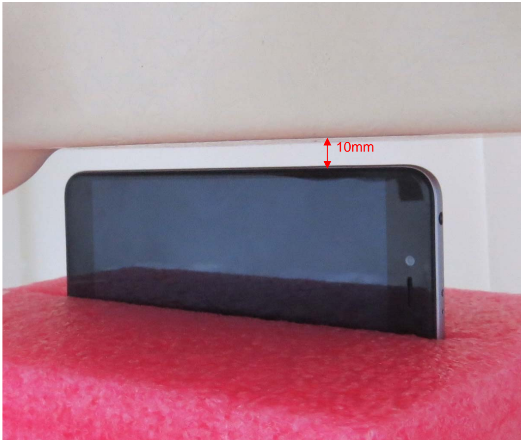
Left Side, the distance from handset to the bottom of the Phantom is 10mm
