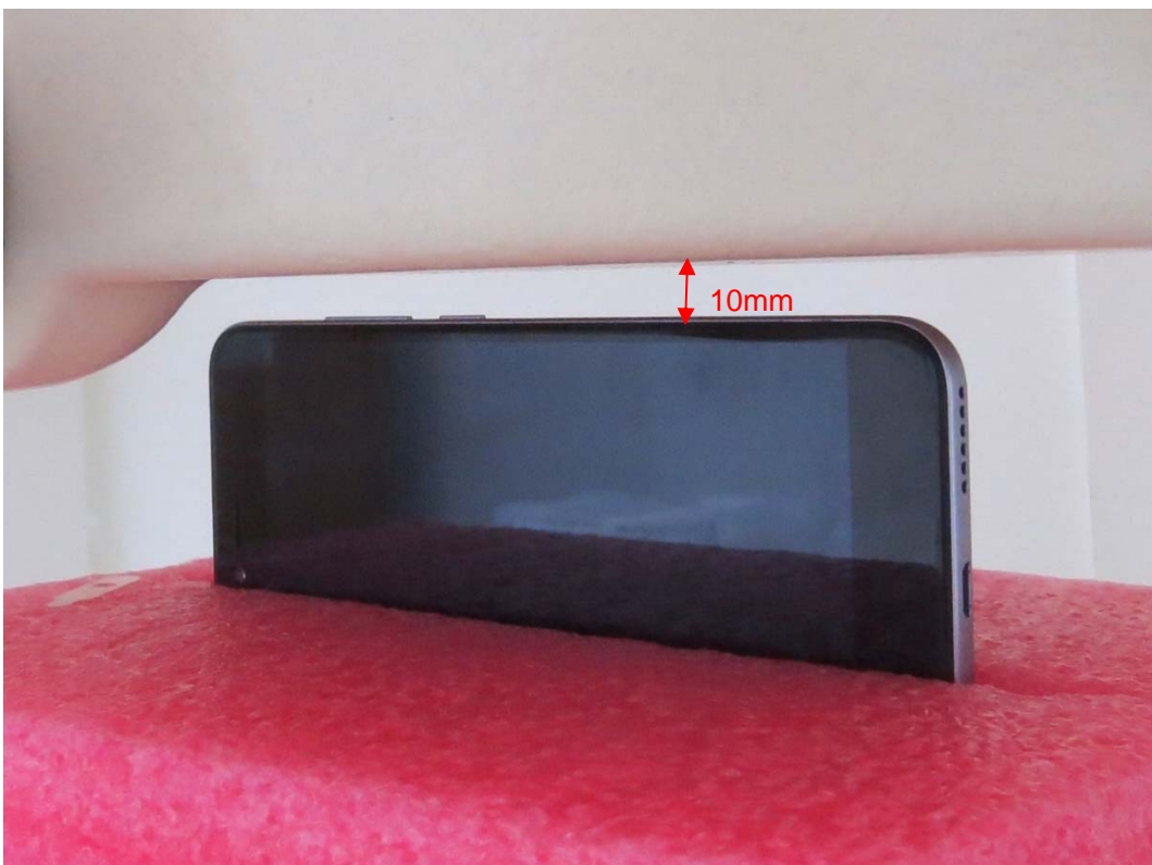
Right Side, the distance from handset to the bottom of the Phantom is 10mm
