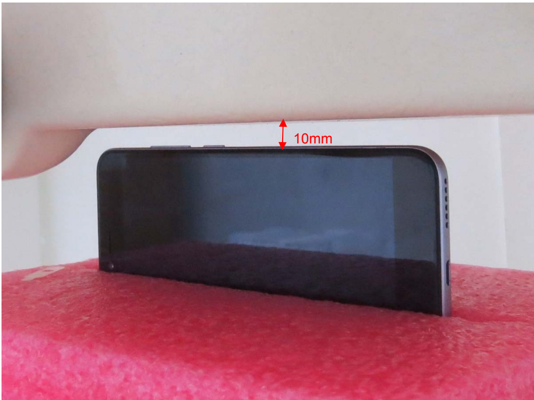
Picture 21: Right Side, the distance from handset to the bottom of the Phantom is 10mm
