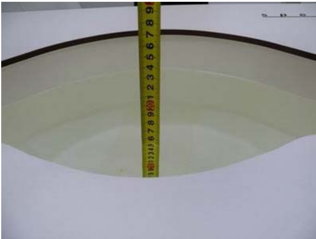
Picture 12: Liquid depth in the flat Phantom (2600 MHz, 15.3cm depth)
