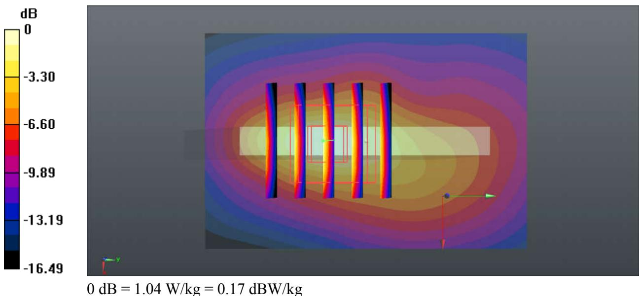
**18\_LTE Band 5\_10M\_QPSK\_1RB0\_25Offse\_Back\_10mm\_Ch20525**
