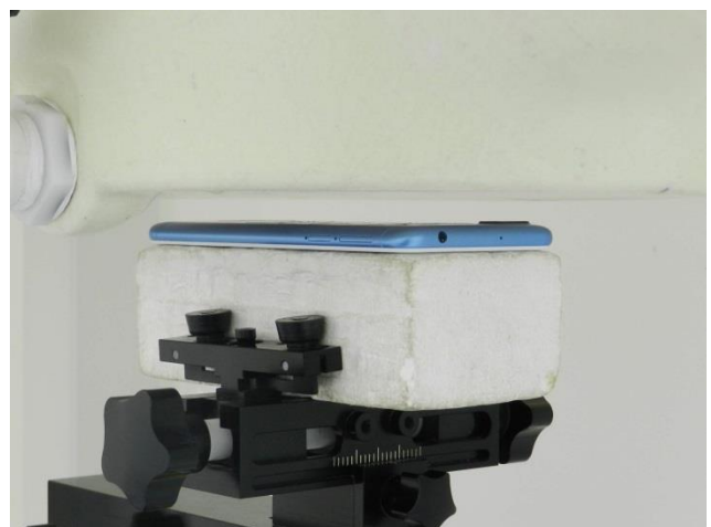
Back, Test Separation 10 mm
