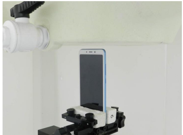
Top Side, Test Separation 10 mm
