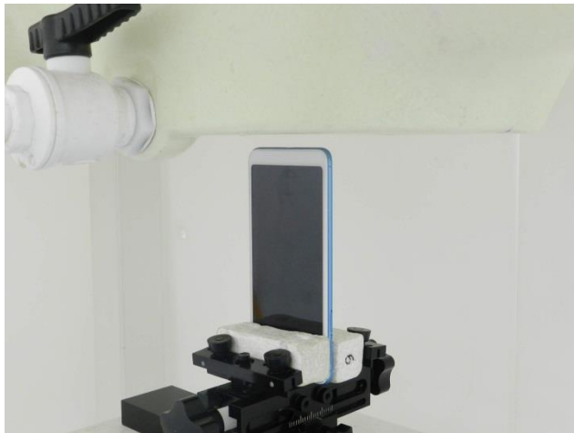
Bottom Side, Test Separation 10 mm
